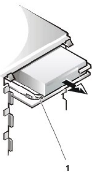
Figure 13. Attaching the Drive Bracket to the New Drive
